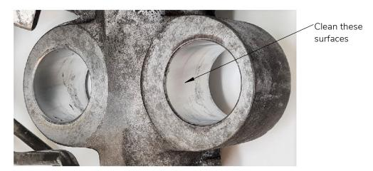
4. Clean the subframe from dirt/oil. Sandblast the subframe if possible.
