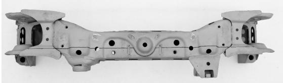
7. Turn the subframe over and position Template\_3 and Template\_4 as shown in picture. Mark the cutting lines. If possible, mark the centre of the arc and drill with a 25mm/1" drill bit. If not, cut it out later with the angle grinder.
