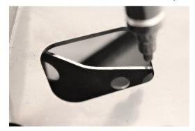
17. Draw an arc from these two points approximately 12mm/ 0.5" deep. Remove the marked section. For LHD cars do this modification to the left side. For RHD cars, to the right.
