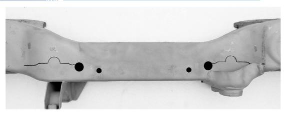
8. Position Template\_7 as shown in the picture. Mark the cutting line.
