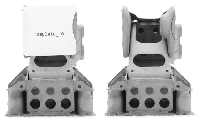
26. Cut the marked section and smooth out any sharp corners. Do this only after welding the subframe.
