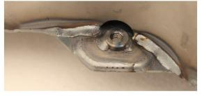
22. If possible, weld the inner walls to the relocation insert from the inside.
