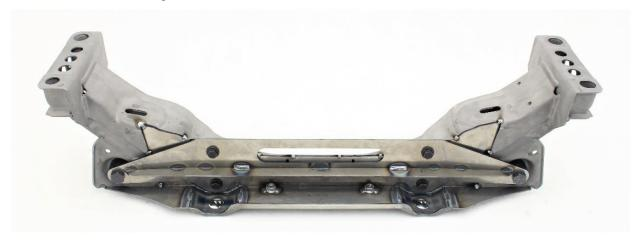
20. Keep the jig in place and fully weld the insert where possible. For extra support, You may temporarily connect the subframe mounts, e.g. with a tube or angle iron. Tube length is approximately 750mm.
