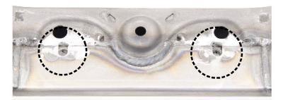
25. Position Template\_10 as shown in the picture. Mark the cutting line. Template\_10 is symmetrical and could be used on both sides of the subframe. The positioning and marking can be done before any cutting or welding.
