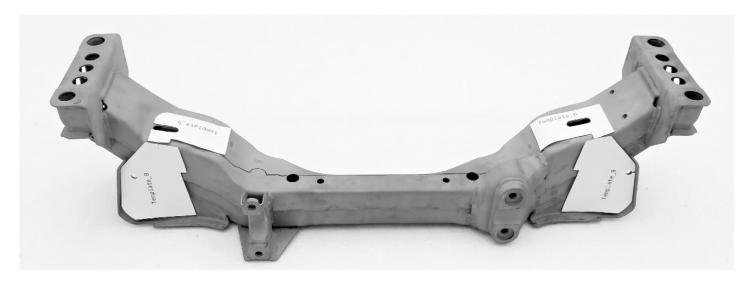
10. Make sure the dotted lines on the templates match each other and mark the cutting line.
