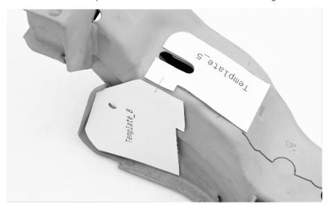
11. Extend the cutting line to the end of the subframe.
