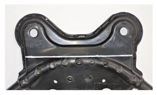
36. To install Wisefab Nissan 350Z Front Drift Angle Lock Kit, the little tabs inside the control arm mounts need to be ground off or pressed flat.
